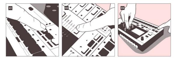
Choose track 1. Make sure the record led is firmly lit and not flashing by pressing the **RECORD** key.
